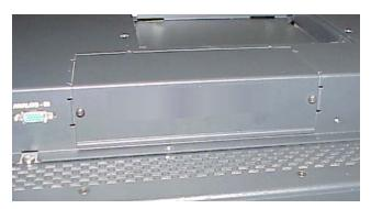
a) Unscrew the two screws holding the blank panel in place. Save the screws for the replacement panel you will install later.
